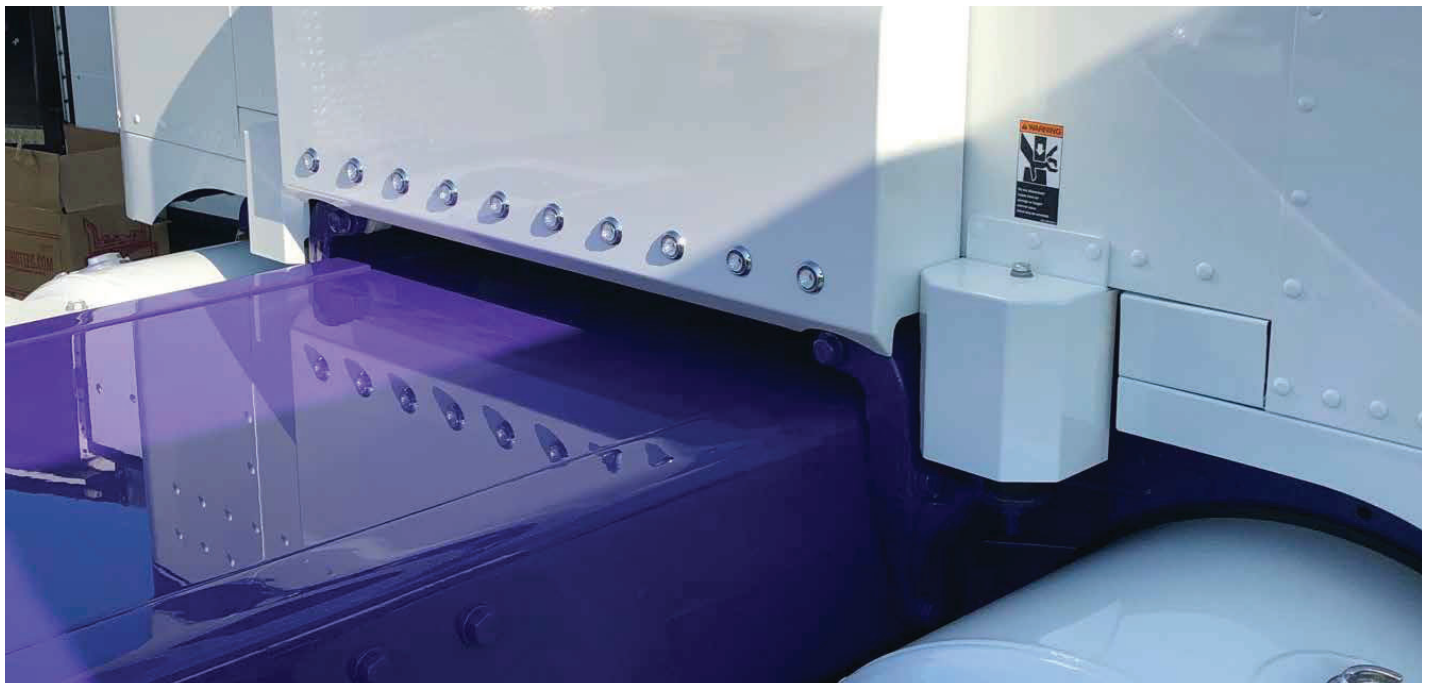
Formed Air Bag Cover (Polished Stainless Steel)
