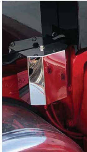
Formed Air Bag Cover (Polished Stainless Steel)
