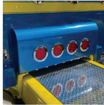
Part Number Example: IC172001-14 - Peterbilt 389 Shock Box Cover with (5) 4" Round Light Holes in 304 #8 Non-Directional Polished Stainless Steel Finish
