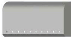
(10) 3/4" light holes on 45 degree face IC172005-21
