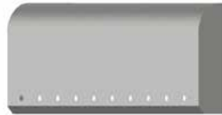
(10) 3/4" light holes on 45 degree face IC172005-21
